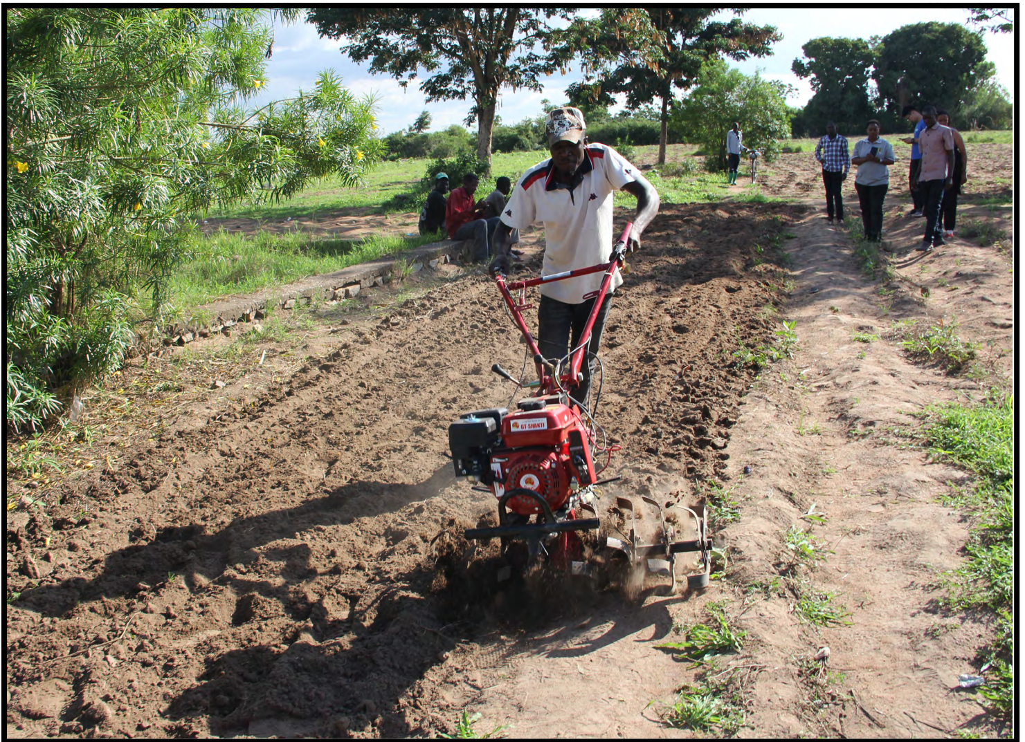
A young farmer demonstrates the use of a power tiller during training in the Kwimba district. Photo: WFP.
